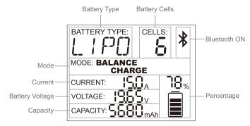
Battery Type: select the chemistry of the battery to be processed.
