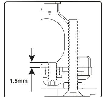
**!** Setting this 1.5mm is a good starting point and will result in a rear droop of 1mm.
