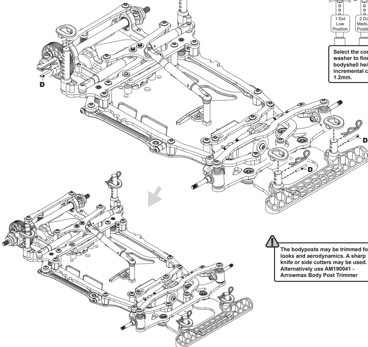
⚠ The bodyposts may be trimmed for looks and aerodynamics. A sharp knife or side cutters may be used. Alternatively use AM190041 - Arrowmax Body Post Trimmer
