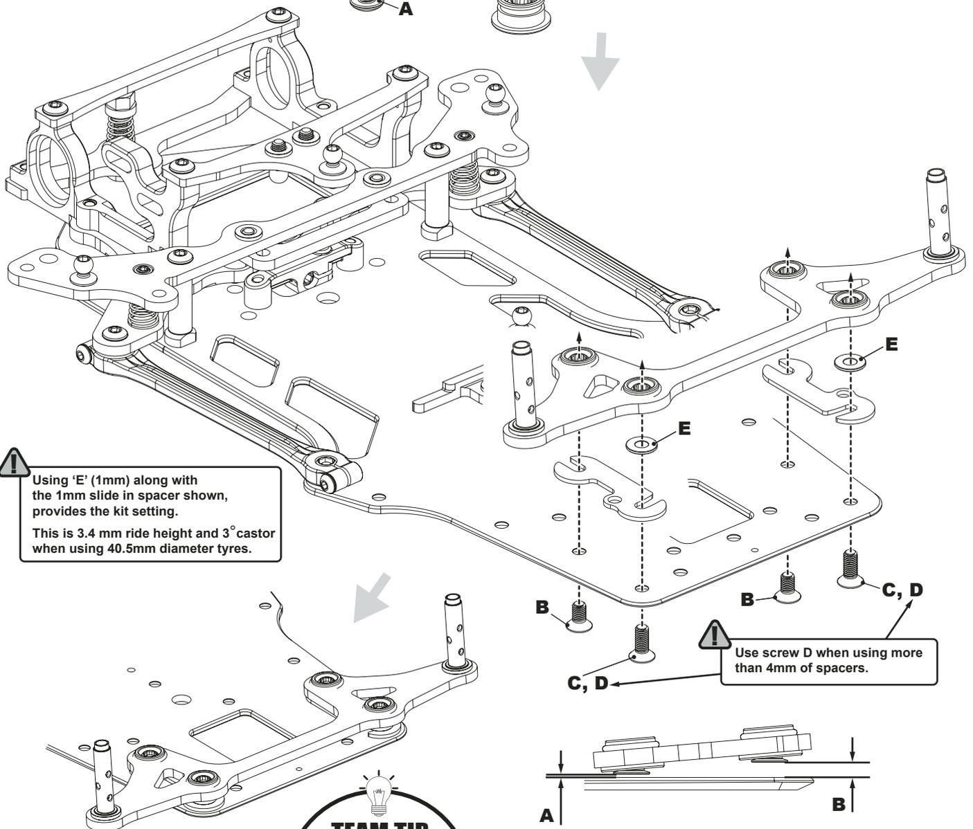
**!** Using 'E' (1mm) along with the 1mm slide in spacer shown, provides the kit setting.
