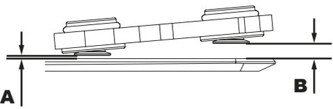
**!** Ride Height and Castor is most easily set with spacers 'A' and 'B'. (as seen in in the diagram above). More information can be found on Page 17.
