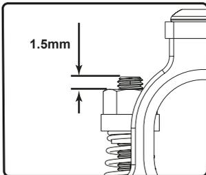
This 1.5mm measurement sets the pod height at the kit setting. The pod base should be horizontal when at ride height.
