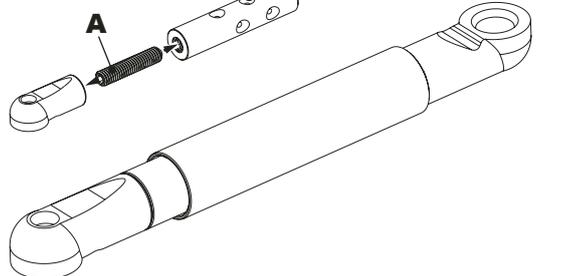
Use the included spanner to tighten the sockets.
