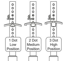
Select the correct body washer to fine tune the bodyshell height. Each incremental change is 1.2mm.
