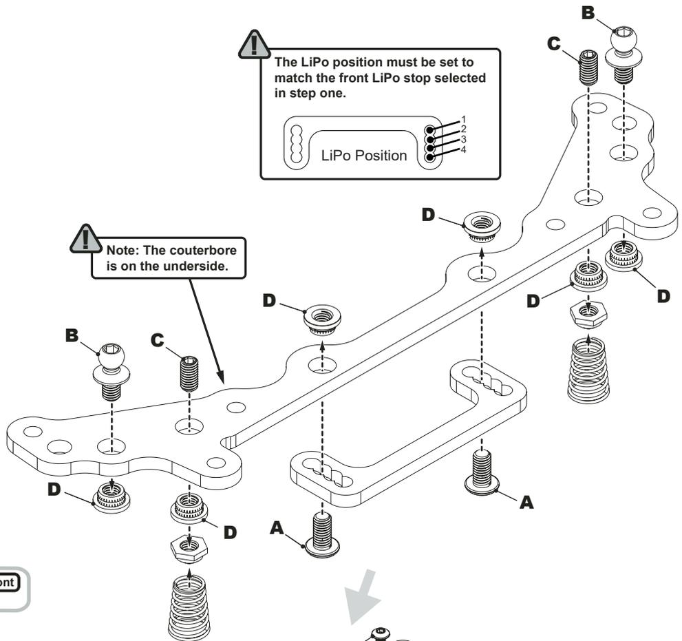
**!** The side springs should be either just touching the lower pod base, or have a small gap. The spring should not have any preload. This is set by adjusting grub screw 'C'.
