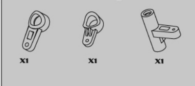
BD2081 Bell Crank Shafts
