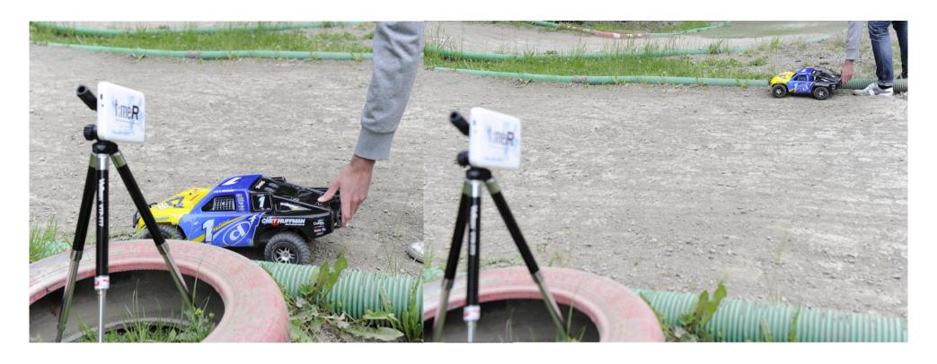
Always do a track test before racing. Sett mini-lap time to 1 sec in LapR then pass the track unit on different positions on the track. Check you hits in LapR. If needed make some adjustment on the track unit or the transponder angle.
